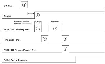
Note: If Normal call processing is enabled (see Programming section C), the FAXJ-1000 will monitor for CNG or touch tones during two 4 second periods instead of only one. If calls intended for the Fax are being incorrectly routed to the Phone 1 port (because the CNG was not detected), enable the Normal call processing mode (\*5). The Normal call processing mode will cause voice callers to hear one more ringback before they ring through to the Phone 1 port.
