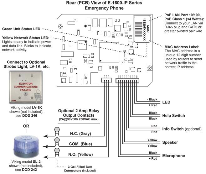
**Note:** The gel-filled (water-tight) butt connectors are designed for insulation displacement on 19-26 gauge wire with a maximum insulation of 0.082 inches. Cut off stripped wire ends before terminating.
