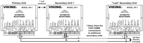
\* Note: The CAN COMM. terminals are polarity sensitive. \*\* Note: To avoid audio ring coupling, space units at least 3.0" apart.
