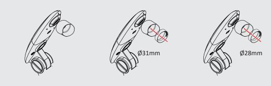
**4.** Mount/remove the microscope adapter onto/off the lens by performing the action shown in the picture below.
