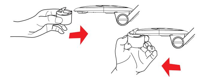
**5.** Connect the lens and microscope adapter to the microscope.
