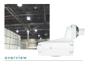
Venture Lighting's outdoor, wet-rated motion sensor utilizes Passive Infrared (PIR) detection technology into a line voltage motion sensor. Designed to mount directly through a 1/2" knockout (7/8" hole) in a light fixture or pole, the sensor utilizes 100% Digital Passive Infrared (PIR) technology that is tuned for walking size motion while preventing false tripping from the environment.
