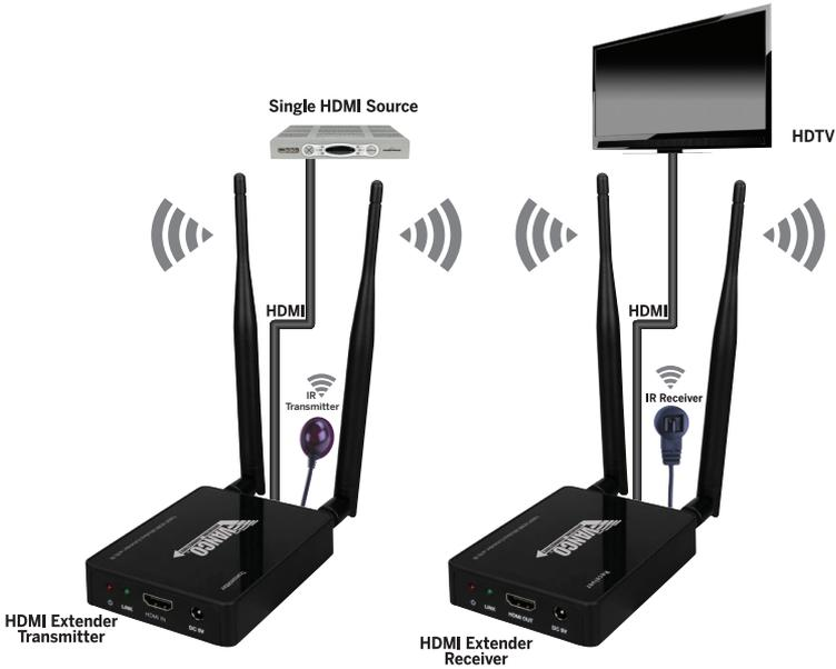
1. Connect the Transmitter to an HDMI source
