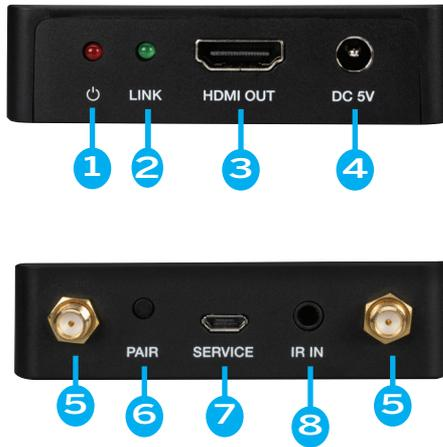
1. Power LED: Illuminates when the Receiver (RX) is powered on
