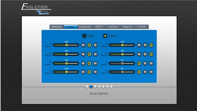
Adjust L+R output audio volume by the volume bar and the three buttons on the right side
