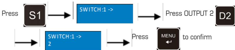
Note: In default status, 4 IR OUT ports correspond with 4 HDMI INPUTS. When you switch an HDMI input, the corresponding IR OUT will be switched synchronously
