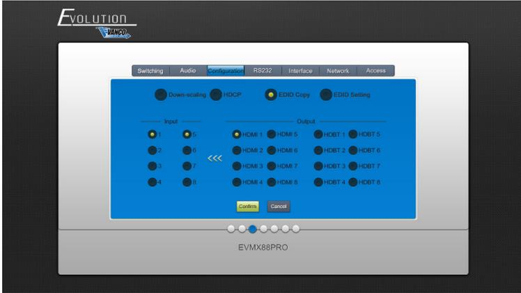
Copy the EDID data from a single output port to one or several input ports
