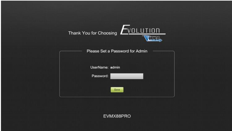
When using the GUI for the first time, an admin password must be set, and then click "Save" to enter the below login tab. Be sure to record the password(s).
