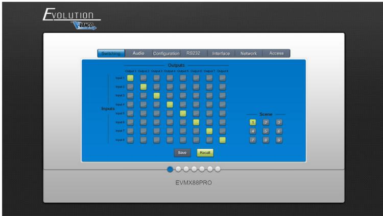
Use the 8x8 button grid on the page to set which inputs are directed to which outputs. For example, clicking the button on the Input 1 row and Output 1 column, directs input 1 to output 1.
