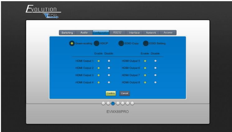
Enable/disable video resolution down-scaling function of HDMI output 1~8 ports.
