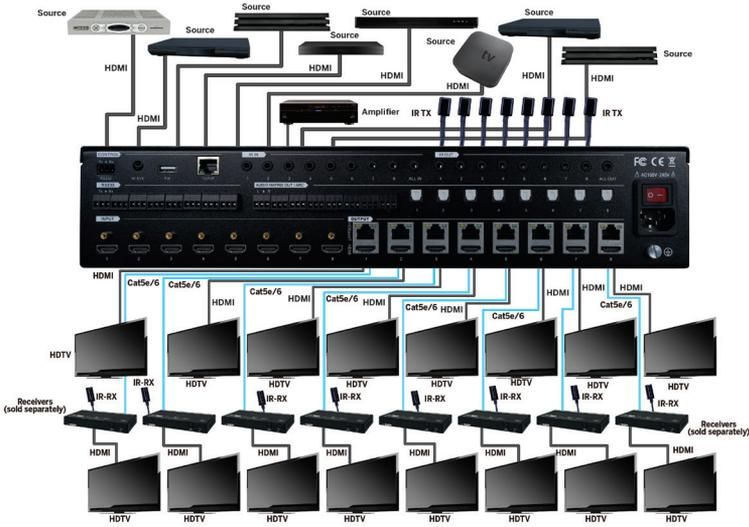
1. Connect HDMI sources to the HDMI inputs of the EVMX88PRO (NOTE: HDMI certified cables are strongly recommended for 4K HDR resolution)
