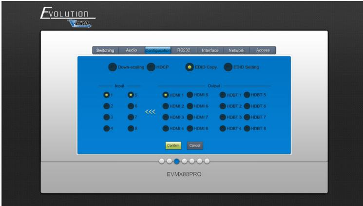
Set the HDCP mode of HDMI and HDBaseT outputs to Passive or Active
