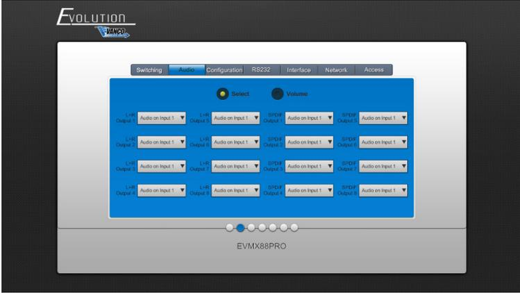
There are sixteen audio sources can be selected for eight analog L+R audio output ports, audio sources can be selected for eight digital SPDIF output ports.
