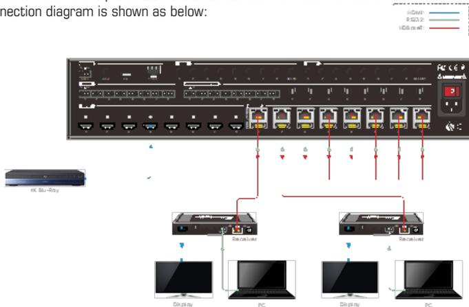
Note: The command "RS232RCMIXION." (IXI=0~8) needs to be sent to enable or disable this control mode. For example, send the command "RS232RCMOON." to enable the remote-control mode for all HDBaseT outputs, and send the command "RS232RCMOFF." to disable the remote-control mode for all HDBaseT outputs. Please refer to the 8.3.1 System Control for more details.
