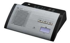
The TS-912 is a Delegate unit with voting function that can be connected to the conference system by a cable. The TS-912 is directly connected to the TS-919B1 or TS-919B4 Bridge unit, then to the TS-910 Central unit via the TS-918 Expansion unit. Either the standard type or long type can be selected for the microphone.
