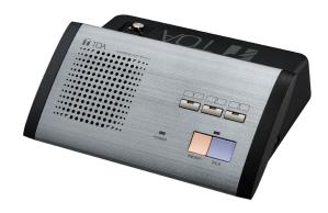
The TS-911 is a Chairman unit with voting function that can be connected to the conference system by a cable. It is equipped with a priority switch, allowing speech to take precedence over the Delegate unit. The TS-911 is directly connected to the TS-919B1 or TS-919B4 Bridge unit, then to the TS-910 Central unit via the TS-918 Expansion unit. Either the standard type or long type can be selected for the microphone.
