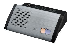
The TS-811 is a Chairman unit that can be connected to the conference system by a cable. It is equipped with a priority switch, allowing speech to take precedence over the Delegate unit. The TS-811 is directly connected to the TS-919B1 or TS-919B4 Bridge unit, then to the TS-910 Central unit via the TS-918 Expansion unit. Either the standard type or long type can be selected for the microphone.
