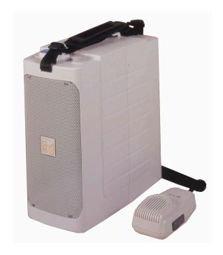
The ER-604W is a compact, lightweight shoulder-type megaphone with whistle signal. It's close-talking microphone has a handy-to-operate volume control and press-to-talk switch. External microphone inputs on the unit's rear panel can accept an optional microphone or a headset microphone for hands-free use. In addition, an AUX (auxiliary) input can accept a CD, MD, or cassette player.
