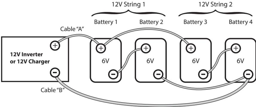
Fig. 7.4: Series-Parallel Connection
