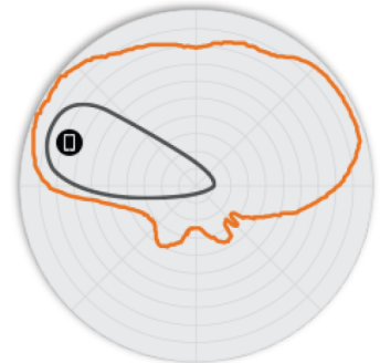
Figure 5. T750 5GHz Elevation Antenna Patterns
