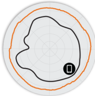
Figure 3. T750 5GHz Azimuth Antenna Patterns
