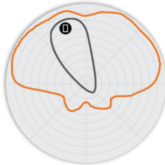
Figure 4. T750 2.4GHz Elevation Antenna Patterns
