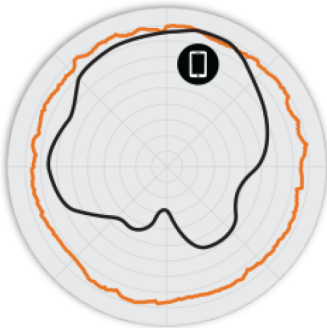
Figure 2. T750 2.4GHz Azimuth Antenna Patterns
