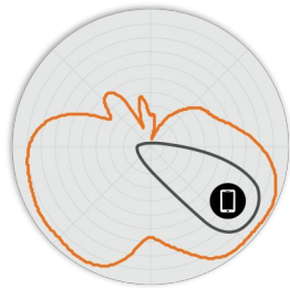
Figure 5. T670 2.4GHz Elevation Antenna Patterns
