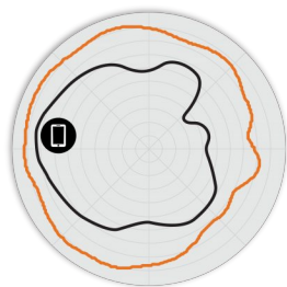
Figure 5. T670 2.4GHz Elevation Antenna Patterns
