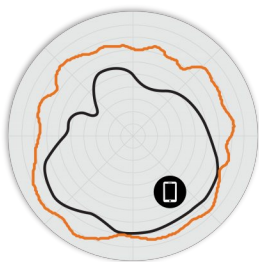
Figure 6. T670 5GHz Elevation Antenna Patterns
