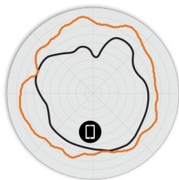
Figure 7. T670 6GHz Elevation Antenna Patterns
