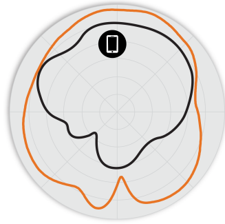
Figure 3. H550 5GHz Azimuth Antenna Patterns
