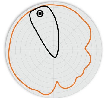
Figure 5. H350 5GHz Elevation Antenna Patterns
