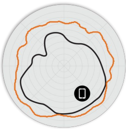
Figure 6. T670 5GHz Elevation Antenna Patterns
