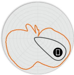
Figure 5. T670 2.4GHz Elevation Antenna Patterns
