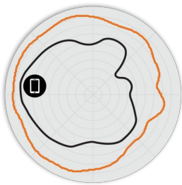
Figure 5. T670 2.4GHz Elevation Antenna Patterns
