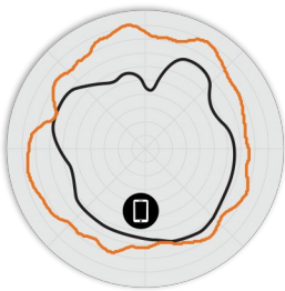
Figure 7. T670 6GHz Elevation Antenna Patterns
