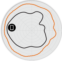
Figure 5. R770 2.4GHz Elevation Antenna Patterns
