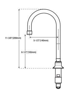
NOTE: All dimensions and specifications are nominal and may vary  $\pm 1/4$ ". Use actual products for accuracy in critical situations. NOTE: The bonnet nut at cold side has a left-hand thread. Turn it clockwise to loosen or counterclockwise to tighten
