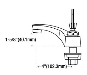
NOTE: All dimensions and specifications are nominal and may vary ±1/4". Use actual products for accuracy in critical situations. NOTE: The bonnet nut at cold side has a left-hand thread. Turn it clockwise to loosen or counterclockwise to tighten
