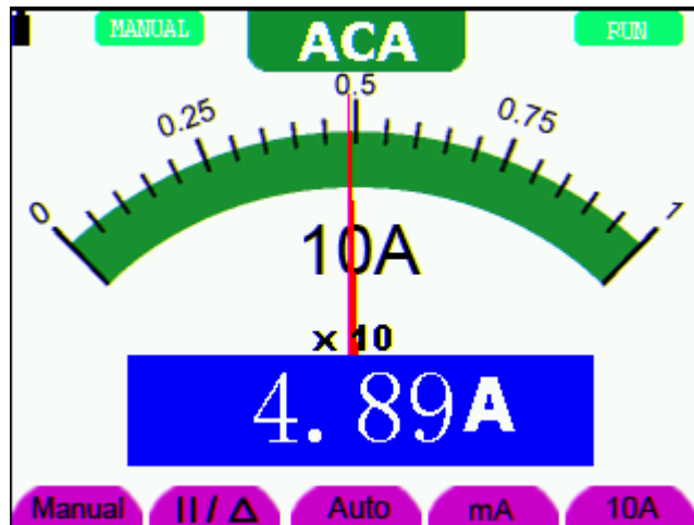
Figure 27: AC Current Measurement for 10A
