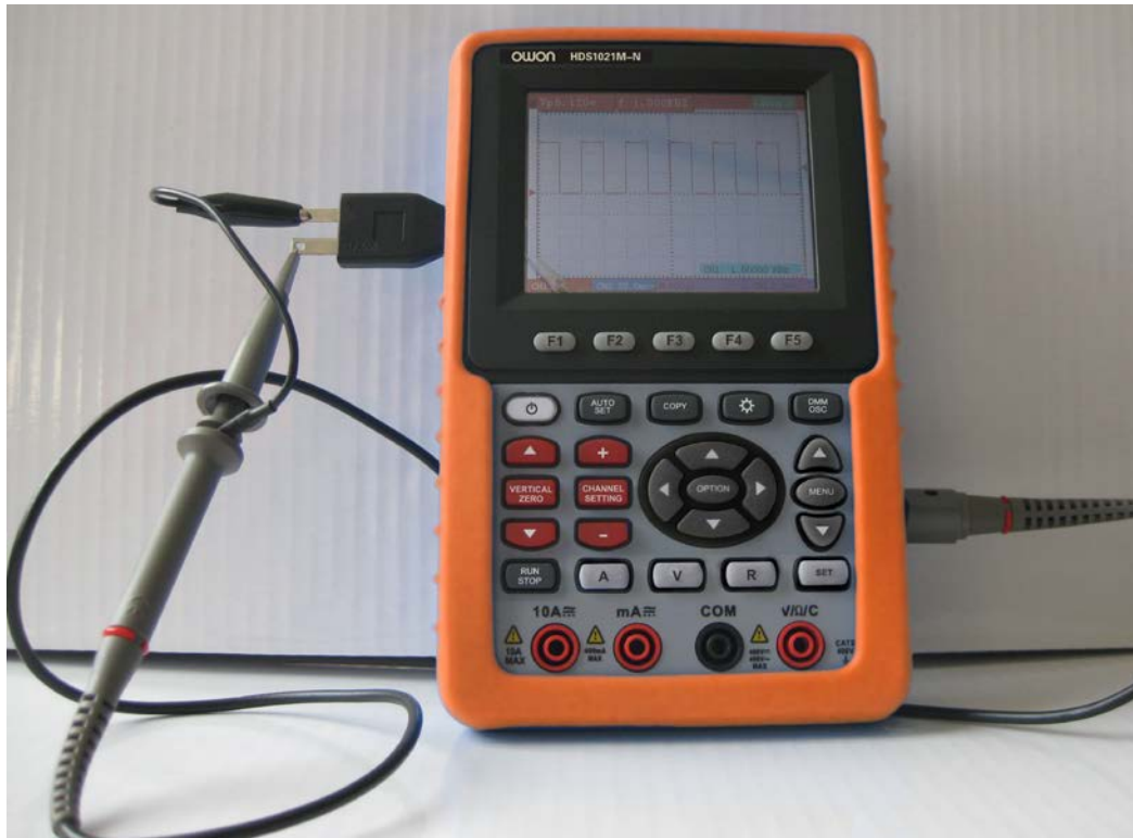
Fig.3. The connection of Square-wave test signal
