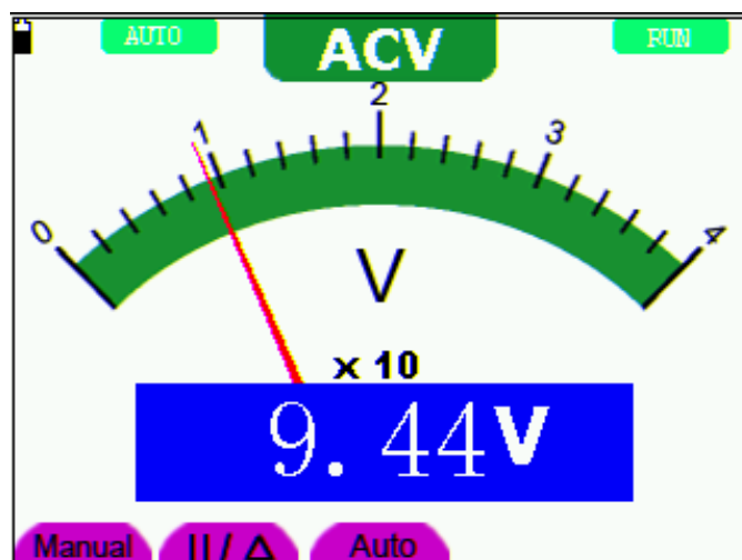
Figure 23: AC Voltage Measurement
