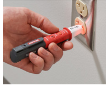
Test wall sockets for AC voltage
