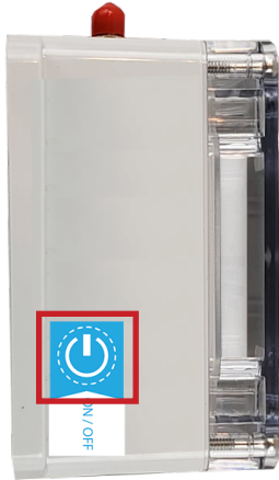
Left side: Magnetic power on/off button
