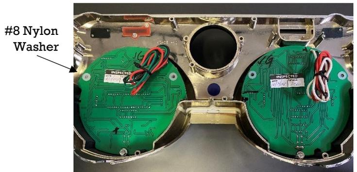
Place 4 of the #8 Nylon washer over the screw holes
