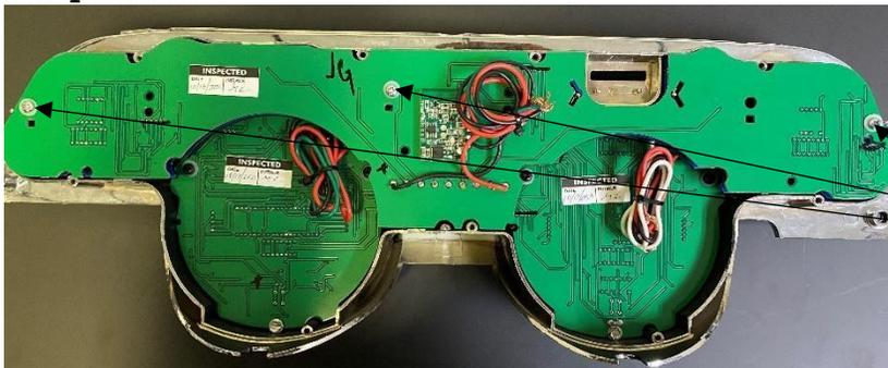
Insert the 3 #6 X 1" panhead screws to secure the instrument board into place
