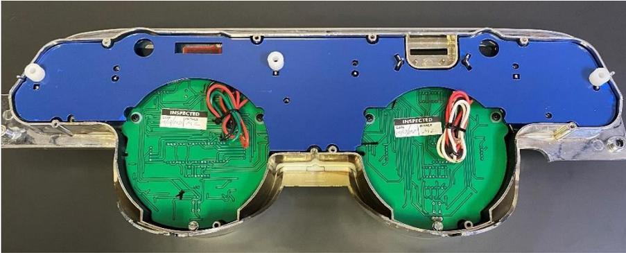
Use the #10 X 5/16" spacers between the lens and circuit board, following the locations pictured
