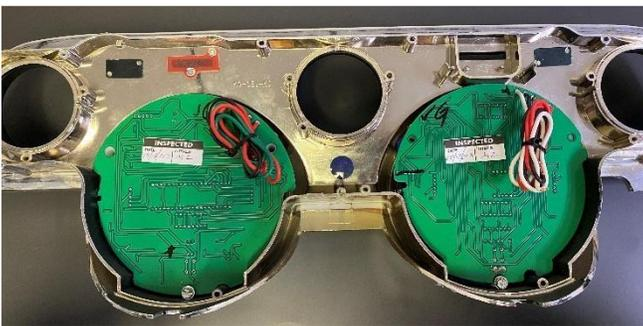
Place the circuit boards into the corresponding locations
