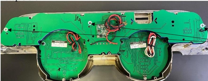
Place the instrument board over the spacers, and place the remaining # 8 Nylon Washers in the location's pictures
