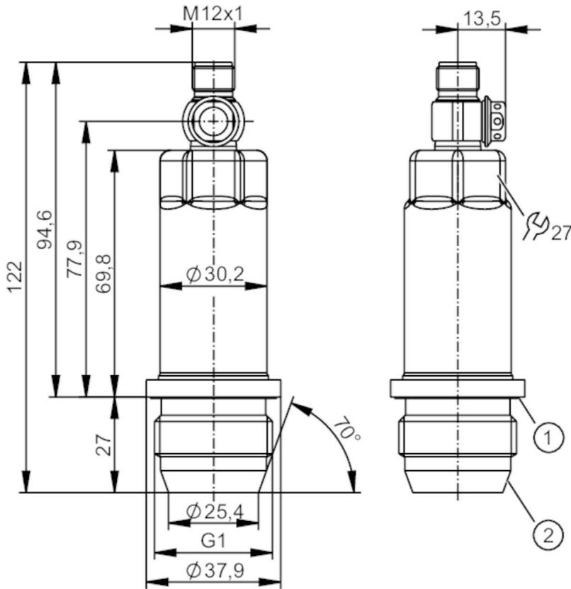
1 groove with sealing ring (DIN EN ISO 1179-2)
