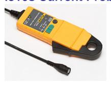
The i310s current probe is based on Hall Effect technology for use in measurement of both DC and AC current. The i310s may be used in conjunction with oscilloscopes and other suitable recording instruments for accurate non-intrusive current measurement.
