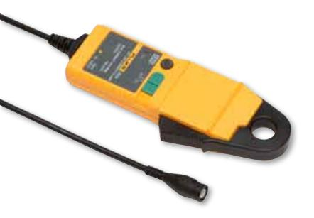
The i30s current clamp is based on Hall effect technology for use in measurement of both dc and ac current. The i30s may be used in conjunction with oscilloscopes and other suitable recording instruments for accurate non-intrusive current measurement.
