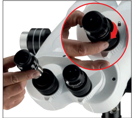
16. Insert and clamp the eyepieces.
