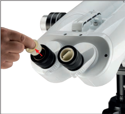
15. Remove the dust caps from eyepiece holder.
