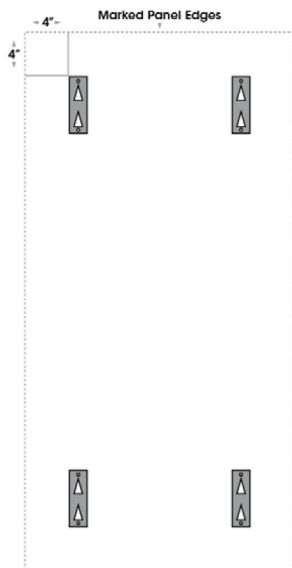
Fig. 1: Front (Standard Impaling Clips Shown) Impaler Placement Planning
