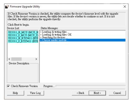
The Utility inspects your installation. All the devices capable of being upgraded by the package are listed in the *Device List* panel.
