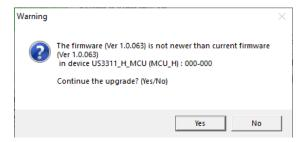
If you enabled Check Firmware Version, the Utility compares the device's firmware level with that of the upgrade files. If it finds that the device's version is higher than the upgrade version, it brings up a dialog box informing you of the situation and gives you the option to Continue or Cancel.
