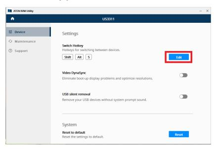
2. The configuration page appears. Click the Device Switch box to configure a new combination of port switching hotkey.
