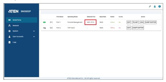
**Note:** The Ethernet port is assigned based on **base socket** settings in *System > General Settings > Service Ports*.
