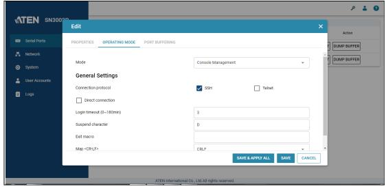
8. Optionally enable the **Direct connection** option if you want to allow direction SSH and/or Telnet connection from the host PC to the connected serial device without going through the SN3002P's console page.
