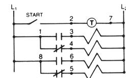
\*For interval operation with a momentary start switch, jumper 2 and 3.
