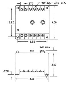
The **SLE Series** is designed to protect 3-phase equipment against **PHASE UNBALANCE**, **PHASE LOSS**, and **UNDER VOLTAGE**.
