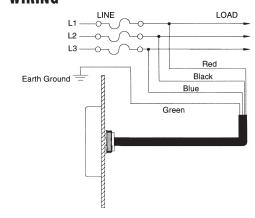
The ATC Diversified Electronics **GFD Series** is intended for the use on ungrounded systems to detect and indicate the phase of the first ground fault condition. This enables corrective action to avoid the potential hazards resulting from a second ground fault.
