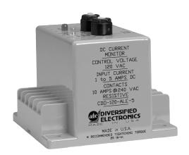
The **CDO Series** is used to detect **OVER CURRENT** conditions. The internal relay energizes (Pick-up) when the monitored current exceeds the preset trip point for longer than the adjustable time delay. The delay is incorporated to prevent nuisance tripping caused by inrush currents. The CDO has an automatic reset feature. The internal relay de-energizes (Drop-out) when the current drops 5% below the preset trip for longer than 0.2 seconds.
