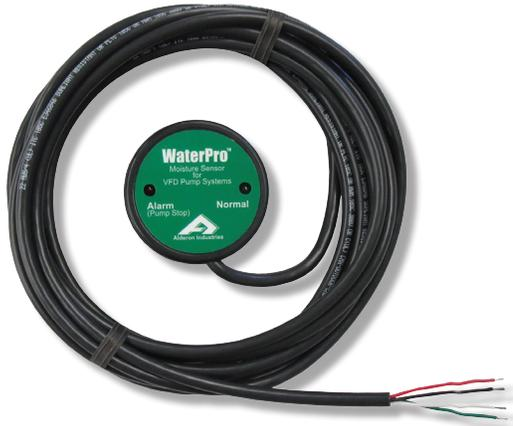
The WaterPro™ VFD Moisture Sensor connects directly to a well or booster pump variable frequency drive (VFD) digital input. The VFD must have a digital input that can be programmed to "fault" or stop the drive and require a manual reset of the VFD to resume normal operation. Available in 12VDC or 24VDC models.
