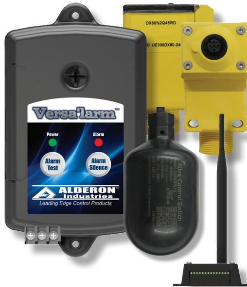
The Versa'larm™ 1-Zone Wireless Alarm System is an indoor rated alarm panel, powered by a standard 120VAC wall outlet. When powered, the green LED will illuminate on the alarm panel. Included with the alarm system: indoor wireless receiver, wireless transmitter, and float switch with optional 47-inch mounting post and 2-inch riser connection kit (riser not included). This alarm system is used for water and wastewater applications.
