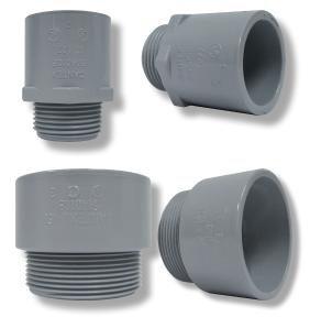
The PVC Hub / Terminal Adapter (male) is typically used with control panel and junction box enclosures to provide a conduit entrance for electrical wiring or cables required per application. Available models include PVC hub sizes from 1" to 2" with a threaded lock nut to securely fasten the terminal adapter.
