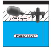
Example 1: If the panel P1, P2, and F1 LED status indicators are illuminated (solid), then the oil layer will be submerging the high water probe.
