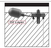
Example 1: If only the panel F1 LED status indicator is illuminated (solid), then the oil layer will be submerging the high water, pump start, and pump stop probes.
