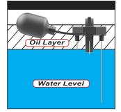
Example 1: If the panel P1, P2, and F1 LED status indicators are illuminated (solid), then the oil layer will be submerging the high water probe.
