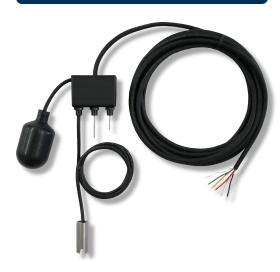
The Oil Alert™ preset level sensor, adjustable probe model, is used with Alderon™ Oil Alert™ control panels for the safe operation of pumping, alarming, and monitoring of: elevator sump pits, transformer vaults, and leachate well applications. The Oil Alert™ control panel will activate a pump to remove water from pits in accordance with ASME A17.1, stopping the pump before oil or other harmful substances enter the water supply.
