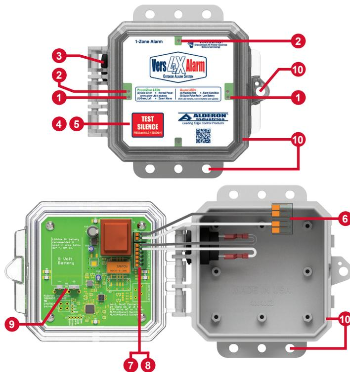
**(1) Power / Zone Indicator LEDs** - Two green LEDs (bottom/middle) illuminate (solid) to indicate the alarm is powered and the left green LED is used as a zone indicator during an alarm condition.
