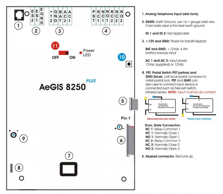
6. LCD Connector Red Line Up. WARNING: If you need to disconnect the LCD's ribbon cable, note down the direction and pins configuration. Connect the LCD's ribbon cable incorrectly, may damage the LCD or board. The RED LINE on the ribbon cable must be connected to pin 1.
