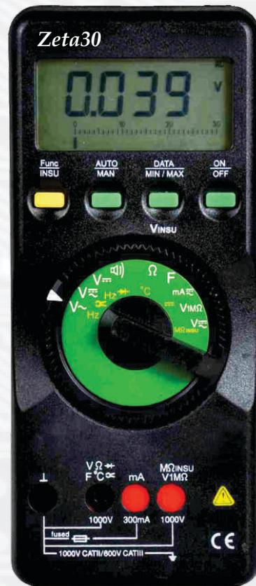
*Zeta 30* is Analog Digital Multimeter with insulation resistance measurement , which measures VAC, VDC, VAC+DC, Frequency, mA DC, mA AC+DC, Resistance, continuity, Diode, Farad, AC current measurement with clip-on sensor and insulation resistance measurement.
