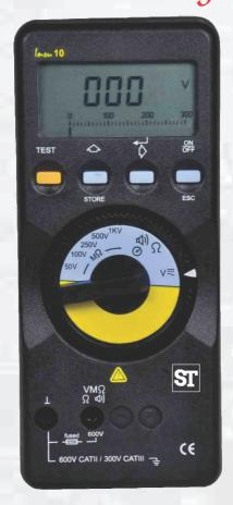
*Insu -10* Analog Digital Insulation & continuity tester for measure of 10Kohm-999Mohm with selectable test voltage upto 1000V. LR measurement from 0.01-99.9 ohm & upto 600V AC/DC. Storage of Min, Max & last 50 readings. Preselectable measurement time, stop watch, fuse blow, auto power off
