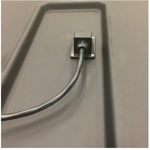
Repeat same steps for next unit (opposite firing), using the other end of the jumper cable. Note: make sure enclosure orientation is correct (opposite facing with correct top/bottom orientation). Once the terminal cover is removed, the terminal will come loose from the enclosure in order to reach the jumper wire.
