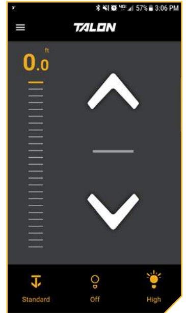
The Talon Control Screen when one Talon is paired to the device. This screen differs slightly when two devices are paired.
