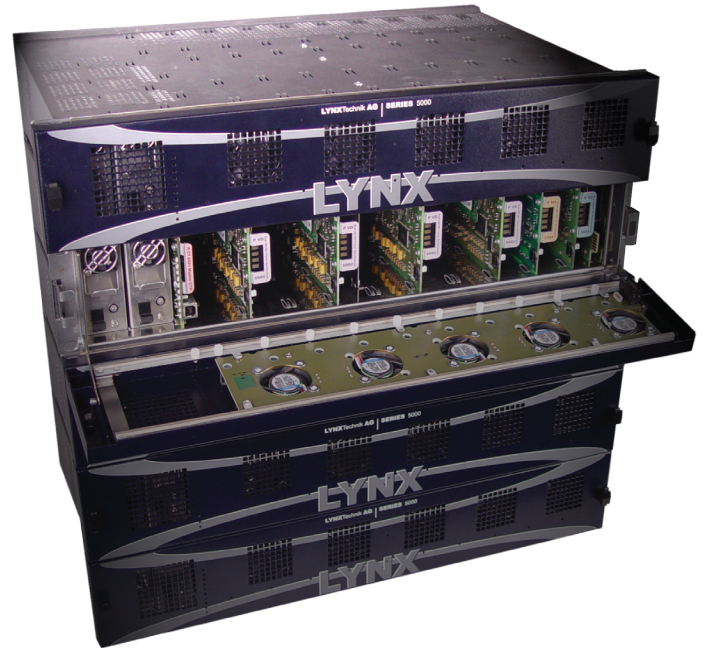
Shows rack front panel hinged open for easy access to all installed devices
