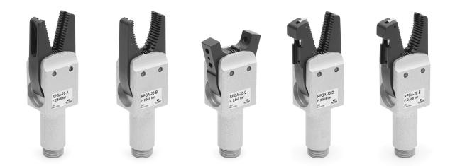
Thanks to a piston with a size of 20mm and to the direct transfer of the force from the piston to the fingers, Series RPGA guarantees a strong and a safe grip. Their technical features ensure a high gripping force and make these grippers particularly suitable in the removal of injection molded items. The surface treatments on each metallic part make this series very wear resistant.
