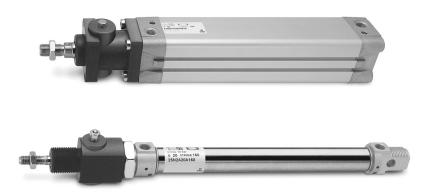
Series RL rod locks are available in 9 different sizes (diameters: 20, 25, 32, 40, 50, 63, 80, 100 to 125 mm). The compact dimensions allow units to be fitted on cylinders where space is limited. Rod lock units are often used to hold the load in position during Emergency Stop conditions or when the air supply may be accidently disconnected from the system. The holding forces are measured at 8 bar and apply in both directions.
